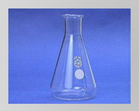
Erlenmeyer flasks hold solids or liquids that may release gases during a reaction or that are likely to splatter if stirred or heated.
