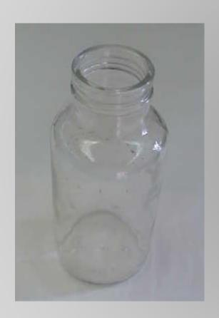
We use gas collecting bottles when large volumes of gases are produced, and must be collected by the displacement of water.
