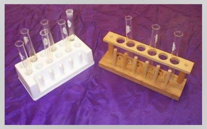
Test tube racks are for holding and organizing test tubes on the laboratory counter. Plastic racks may melt in contact with very hot test tubes.
