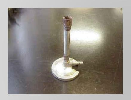
Bunsen burners are used for the heating of nonvolatile liquids and solids.
