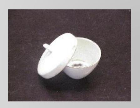
Crucibles are used for heating certain solids, particularly metals, to very high temperatures.
