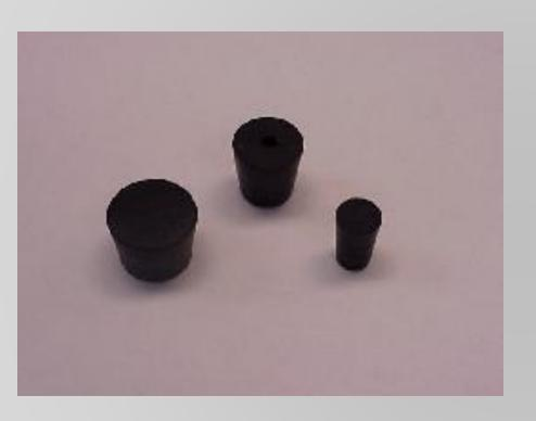
Rubber stoppers are used to close containers to avoid spillage or contamination.
