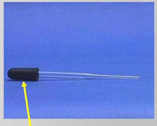
A medicine dropper is used to transfer a small volume of liquid (less than one mL).
