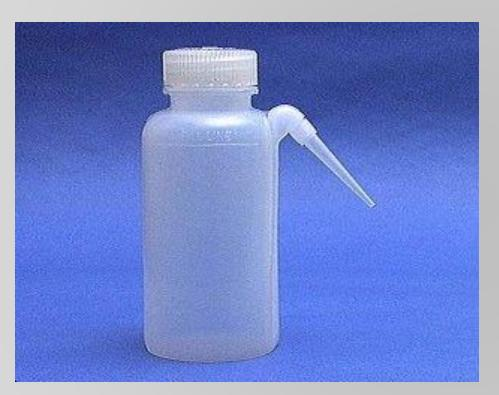
A wash bottle has a spout that delivers a wash solution to a specific area. Distilled water is the only liquid that should be used in a wash bottle.
